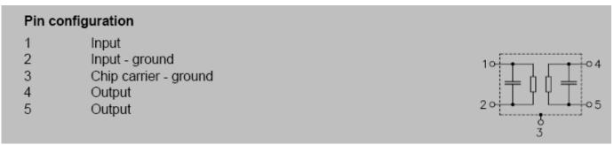
Figure 6.9.2: Pin configuration of X696M
